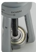
• Adjust the jaws by turning the screw
